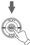
3. Press the [PLAY] or [STOP] button to select [REC MODE], then press the [REC] button.
