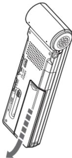
2. Insert the supplied alkaline battery.
