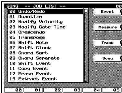
3. Move the cursor to the job you want to execute, or else enter the job number using the numeric keypad. Then press  $\downarrow$  to open the job-execution screen.
