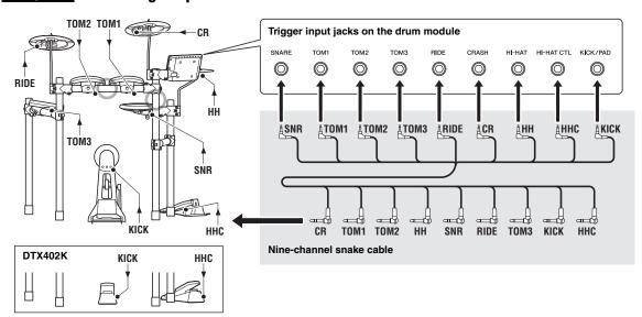
Insert the mini plugs\* at one end of the nine-channel snake cable into the correct trigger input jacks (SNARE to KICK/PAD) on the drum module. (\*: The smaller set of plugs.)
