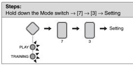
You can set whether the USB audio input is sent to the USB out or not. When set to "Output," the audio data input from a PC (for example) is mixed with your pad performance and they are sent together to the USB out. When set to "Not output," only your pad performance is sent to the USB out, even if the audio data is input and played from the PC.
