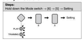
For Dynamic Gate (page 33), you can set the low limit (the threshold value between "Weak" and "Normal").
