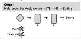
You can set the [PHONES/OUTPUT] jack to output either mono or stereo sound. We recommend that you select the Mono setting if connecting a standard mono-audio cable to this jack in order to use your drum module with external speakers, a mixer, or other similar equipment.
