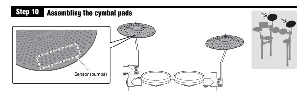
The crash cymbal, which has the sticker labeled "CRASH" on the rear side and has some bumps on the front side, is for the **left**.
