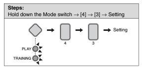
You can adjust the position at which the hi-hat switches from open to closed when you operate the hi-hat controller. The lower the value, the smaller the virtual opening between the top and bottom hi-hats. Larger values increase the size of the gap between the top and bottom cymbals, and this can prevent foot close or foot splash sounds from being produced when you operate the pedal.
