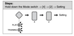
You can set the degree of sensitivity for detecting hi-hat foot splashes. The higher the value, the easier it will be to produce a foot-splash sound with the hi-hat controller. High values may, however, result in splash sounds being unintentionally produced when, for example, you operate the hi-hat controller lightly as you keep time. It is a good idea, therefore, to set this parameter to "Off" if you do not want to play foot splashes.
