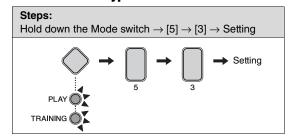
You can specify the type of snare pad connected to your drum module.
