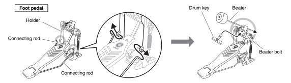
**5.** Turn the foot pedal's T-bolt counter-clockwise to loosen it.
