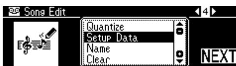
**10** Press the [NEXT] button to display the SETUP DATA screen.
