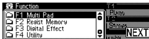
In this case you can select the desired function by turning the **data dial** or move the cursor by pressing the [+ / YES] / [- / NO] buttons.
