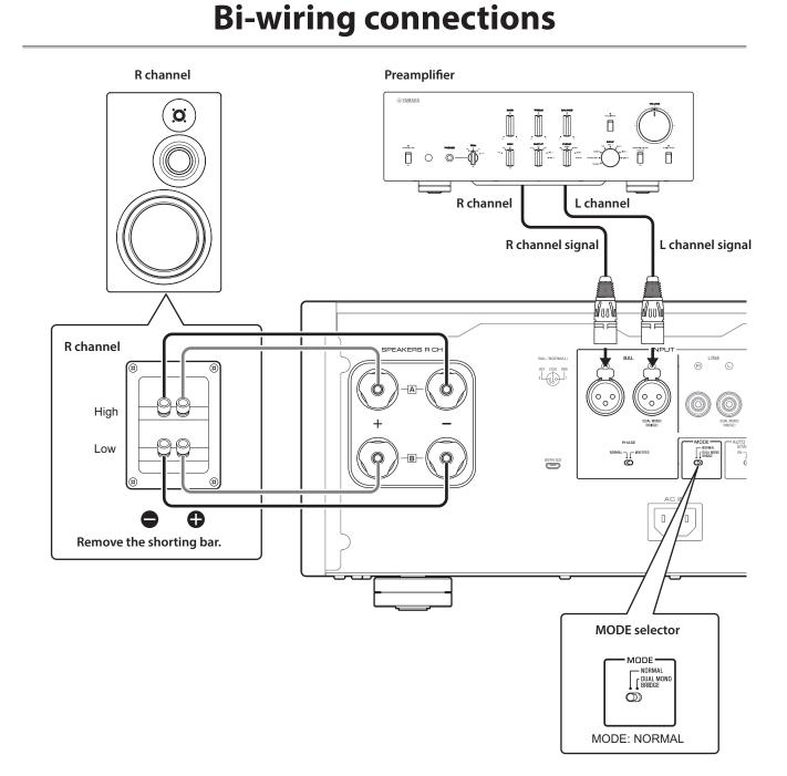
To bi-wire your speakers, separate cables are used to connect the mid/high-frequency speaker driver (tweeter) and the low-frequency driver (woofer) on each biwireable speaker to the amplifier. Running separate cables from the amplifier can have a profound impact on relieving the tweeter circuit from the back flush of EMF (electromotive force) generated by the woofer's voice coil, resulting in less interference between HF and LF ranges and better sound quality.
