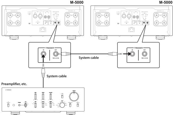
To control the unit in a trigger connection configuration, set the STANDBY/ON/OFF (Power) switch to STANDBY/ON.
