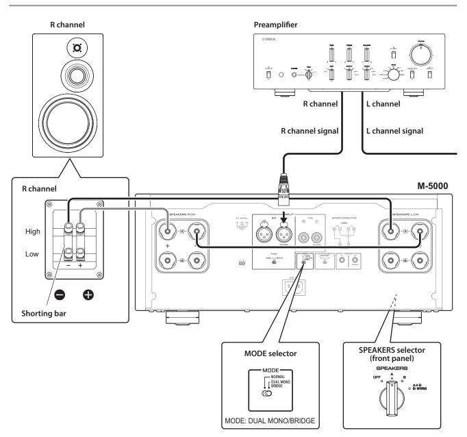
In a bridge connection configuration, the M-5000 is used as a monaural amplifier. To create a stereo system, you need two M-5000 units.
