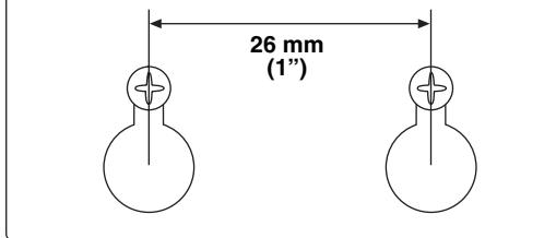
Fasten screws into a firm wall or wall support as shown in the figure below, and hang the holes on the protruding screws.
