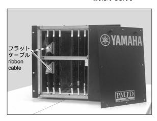
2. Remove eight fixing screws on the rack mount hardware, and remove the rack mount hardware. Do not remove any screws or hardware other than those shown in the picture.
