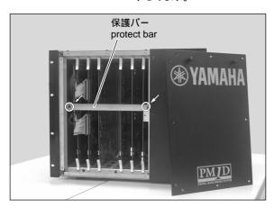
**4.** Lift up the protect bar and remove it.
