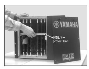
5. If you are replacing the PDB1D board and the GDB1D board, remove two connecting ribbon cables.
