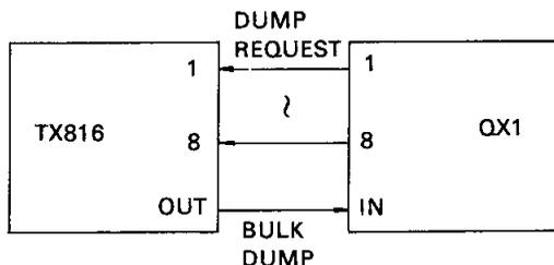
With your system set up as shown in the above diagram, specify the bulk number and slot number, then press **ENTER**. Then, following the QX1 prompts, set the OUT SLOT on the TX816, then press **ENTER** on the QX1. This will initiate bulk data transmission from the TX816 to the QX1. This operation is repeated for each slot, following the slot numbers displayed by the QX1.
