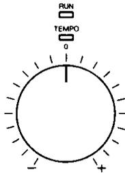
Changes the tempo during playback or record. This change is temporary and does not affect the programmed tempo. The new tempo setting is indicated on the LCD.
