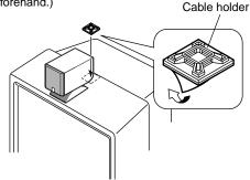
2 Tie the speaker cable to the holder firmly with a provided vinyl-coated wire (which is originally used for bundling the speaker cables) as shown below.
