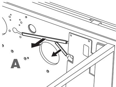
**6-2** Align the pedal power cords (that come out from the pipes of D) along with the grooves on the bottom surface of A.
