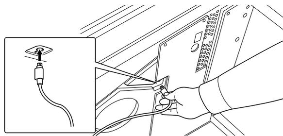
**7-2** Connect the power cord plug to the power connector in the correct orientation.
