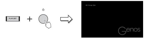
You cannot operate the instrument while in the USB Storage Mode.
