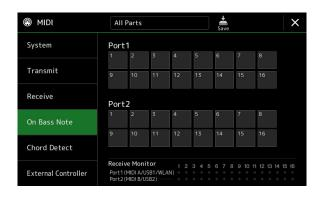
Touch the desired channel number to enter the checkmark. Touch the same location again to remove the checkmark.
