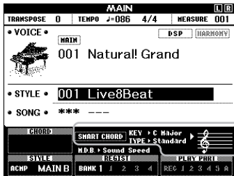
Indicates the current Smart Chord settings, KEY and TYPE when the Smart Chord is on.
