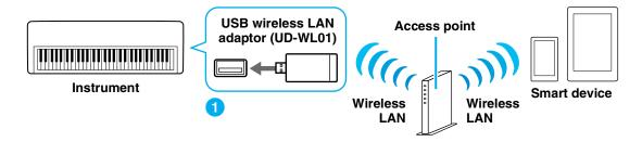
If the wireless LAN function is included on the instrument, skip steps 1 and 2 below.
