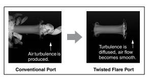
Air turbulence on both ends of the port creates noise
