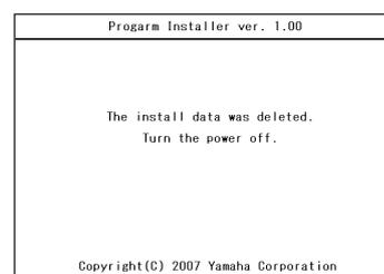
The upgrade data has been deleted from the USB device. Turn off the power switch of the instrument and remove USB device.
